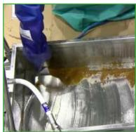
Scoop out remaining debris from tub& wipe down. Iftub is washed, dry thoroughly. Place filter back in tub
