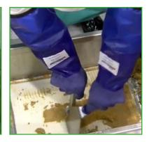
Detach suction hose from riser tube. Scrape debris from filter into tub, remove and set aside. DO NOT GET **FILTER WET**
