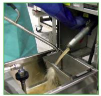
Turn fryer OFF, attach drain pipe, roll filter machine under drain pipe, slowly open drain valve
