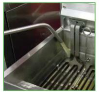
With return wand positioned in fry pot, turn filter pump ON. Wash debris from pot & use poker rod to remove any clogs. Turn filter **pump OFF**
