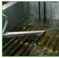
Position return wand in fry pot. Turn filter pump ON. Pump until bubbles appear. Turn filter **pump** OFF. Turn fryer ON
